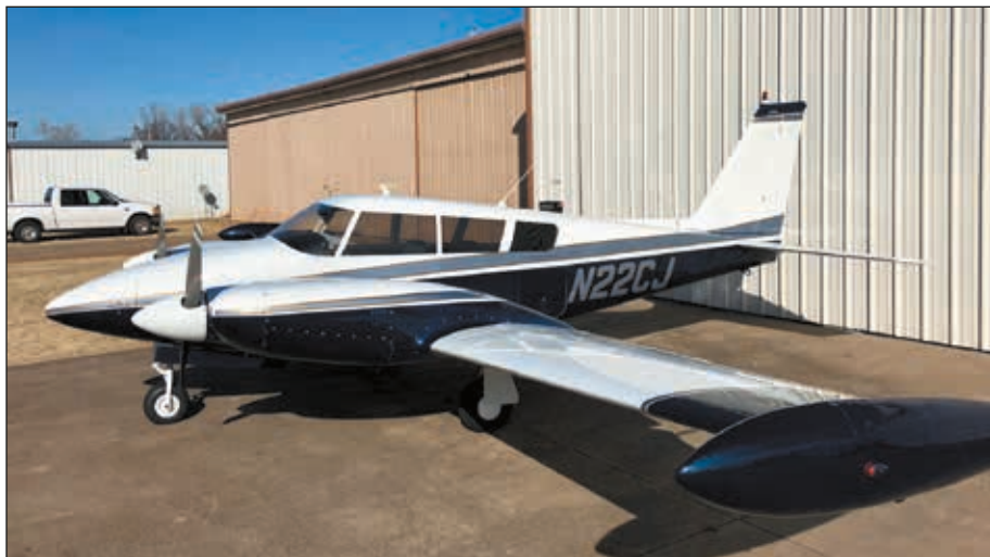
That's Len Duncan's PA-30B. It has RayJay turbochargers and he reports 175 knots at 17 to 18 GPH when flying in the teens.
