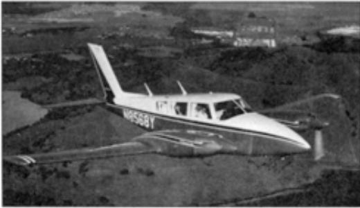
The PA-30C Twin Comanche came next. It, too, has the third side windows and six seats. Better soundproofing and more standard features give this airplane a 60-pound empty weight increase over the earlier non-turbocharged Twin Comanches. The C model also brought with it a more modern panel design and the first appearance of the standard-T presentation of flight instruments. The 120-gallon fuel system with tip tanks was an option. New, the Cs sold for \$52,725.
